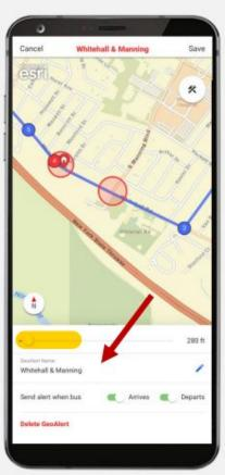
Move the map to position the GeoAlert circle a few minutes away from the stop, use the slider to increase the size, and select when to receive the phone notification
